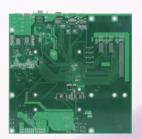
Portwell's 1st COM Express® Rev3.0 Type 7 Carrier which supports four 10GbE optical and fiber phys, NC-SI interface and up to 32 PCI Express lanes.
