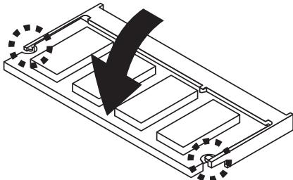
3. To uninstall the DIMM, flip the slot levers outwards and the DIMM will be released instantly.
