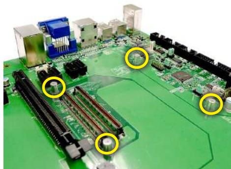
2. Position the module board on top of the carrier board with its mounting holes aligned with the standoffs on the carrier board and the COM Express connectors of both boards aligned to each other. Press the module board down firmly until it is securely seated on the COM Express connectors of the carrier board.
