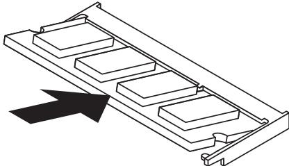
2. Push the DIMM gently downwards until the slot levers click and lock the DIMM in place.
