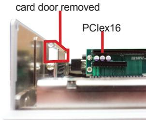
5. Plug the PCI Express card to the due slot. Re-fasten the screw to fix the card in place.
