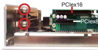
4. After the screw is removed, dismount the card door from the I/O bracket.
