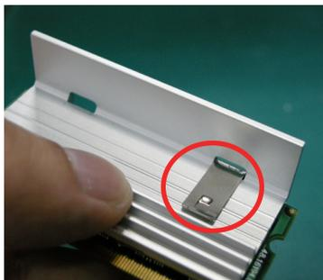
Note: The above mentioned demonstrated one clip only. When you install the memory module with heat spreaders, be sure to use both clips.
