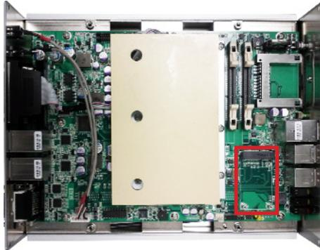
The MiniCard socket's connector has a break.
