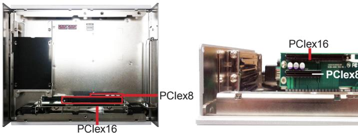
3. Loosen and remove either of the screws as marked in the illustration below depending on which PCI Express slot to use, the PCIe x8 or PCIe x16.
