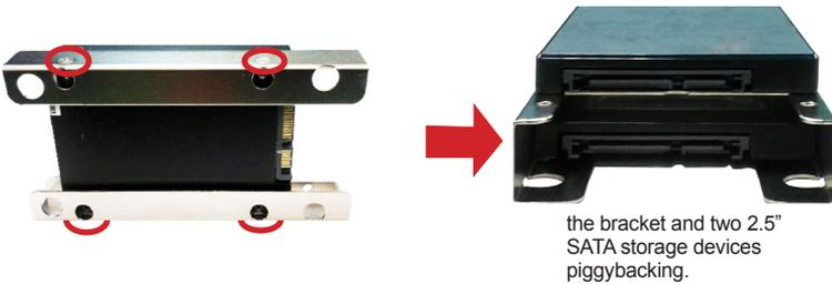
7. Reinstall the bracket (with the storage devices) to the computer.
