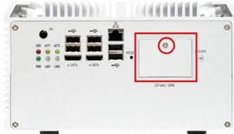
2. Once the screw is removed, open the door. The SIM card slot then comes to view.
