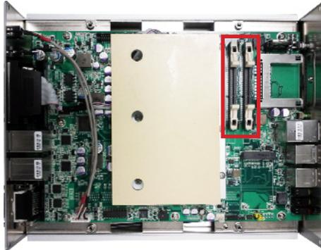
The SO-DIMM sockets are vertical type, and each socket has two latches to fix the memory modules. The memory module can only be installed by one direction due to the key notch.
