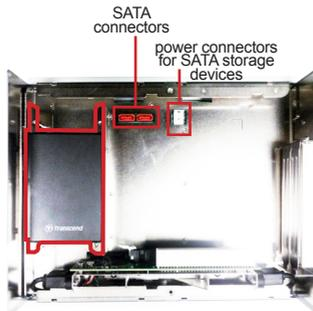
8. Connect the SATA signal cable(s) and power cable(s).
