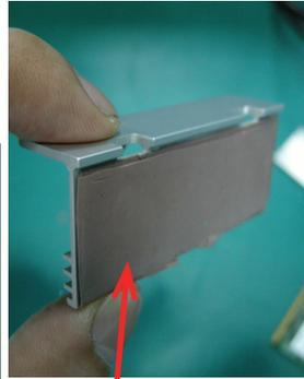
Each heat spreader comes with a thermal pad.
