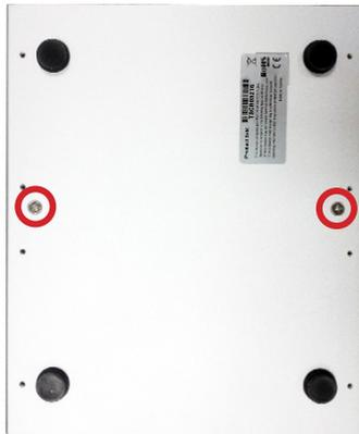
2. From the front panel, loosen and remove the 2 screws as marked in the illustrations below.
