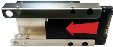
6. Fix another storage device in place by using screws at the four screw holes on both sides of the bracket.
