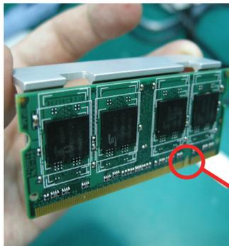
Attach the memory module to the thermal pad
