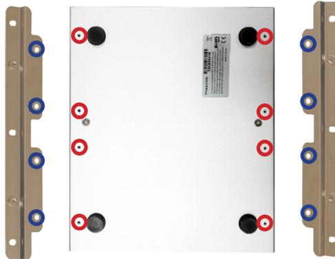
2. Have the two wall-mount brackets. Use the screws included in the wall-mount kit to assemble the brackets to the computer's bottom by the screw holes on them (as marked in the blue circles in the illustration above).
