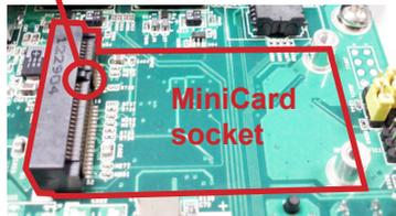
3. Plug a wireless module to the socket's connector by a slanted angle. Note the notch on the wireless module should meet the break of the connector.
