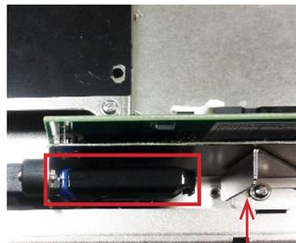
Adjust this iron to make space for the USB drive installed.
