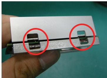
4. Have the two metal clips. Use them to hold the heat spreaders and the memory module together.
