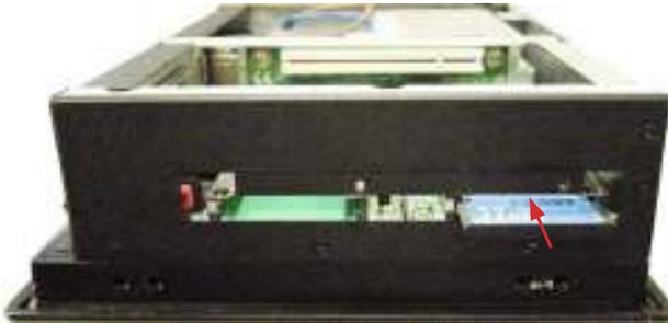
3. If later it is needed to remove the CFast card, simply remove the card door and push-eject the CFast card.
