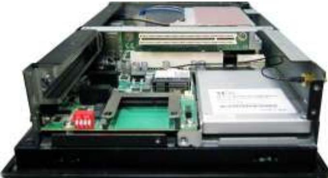
2. Insert your desired PCI card into the slot and fix it in place.
