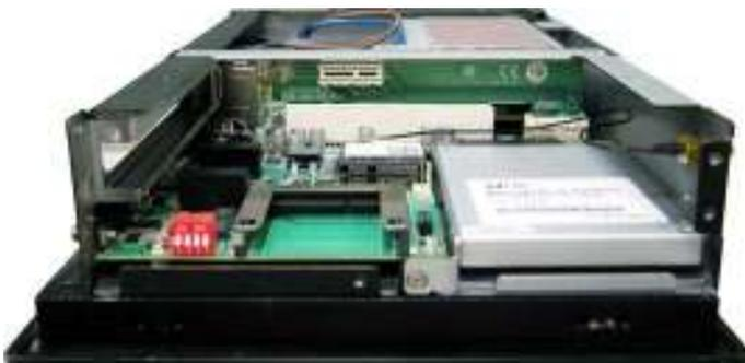
2. Insert your desired PCIe x 1 card into the slot and fasten it.
