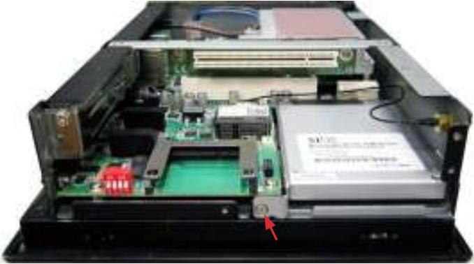
6. The SSD barcket is one of the standard accessories included in the accessory box. This SSD bracket can be replaced by an additional CFAST socket bracket.
