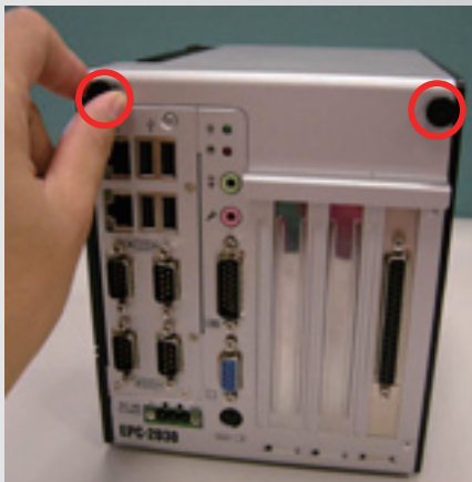
Thumbscrew Design for Easy, Tool-free Installation
