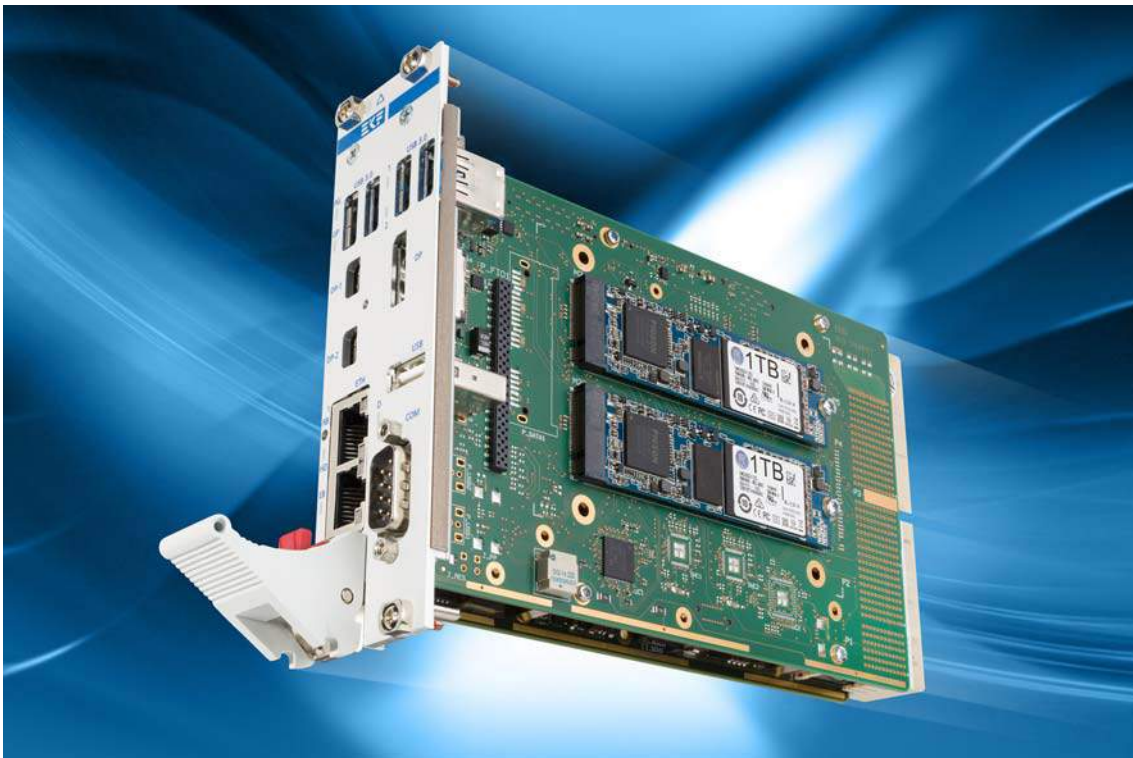
8HP Assembly w. SCS-TRUMPET Side Card & Dual M.2 SATA SSD
