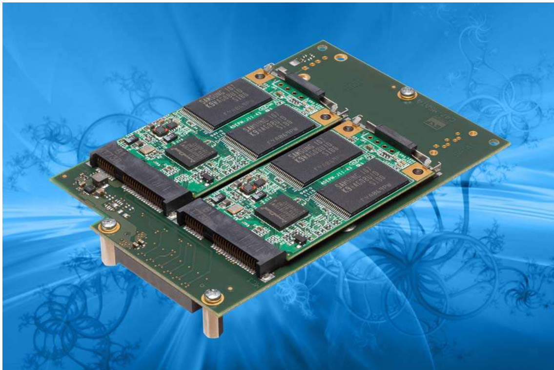
C47-MSATA • Low Profile Dual-SSD Mezzanine Module
