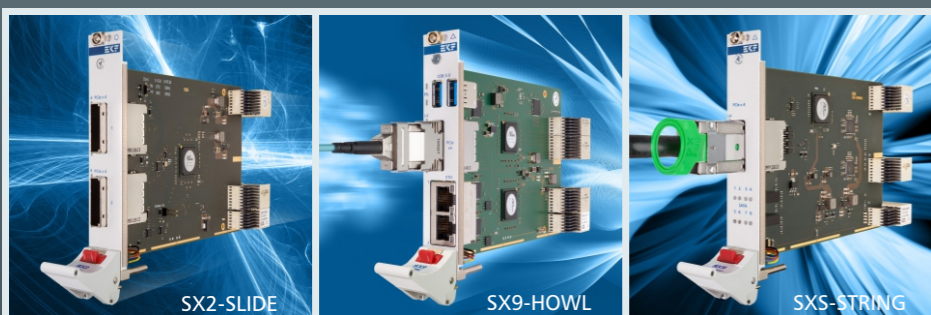
PCIe External Cabling
